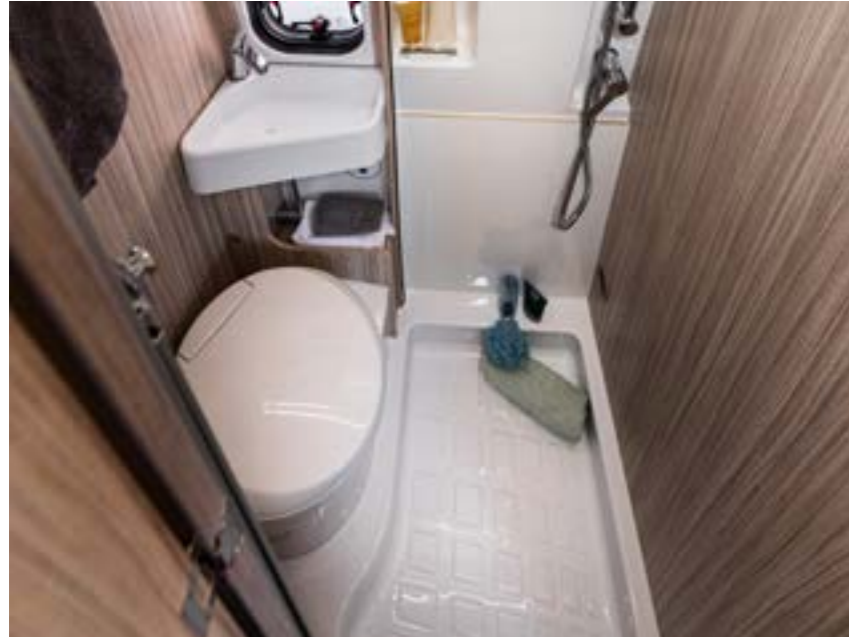
Lowered shower tray: the water does not flow into the toilet area.
